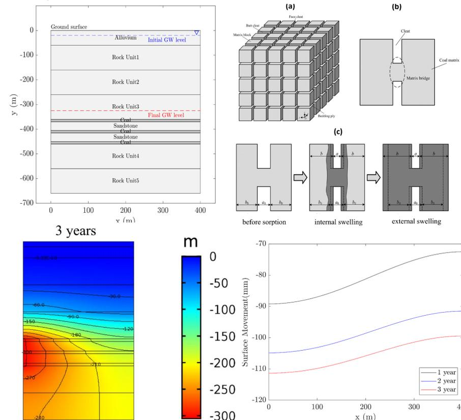
**Figure 2:** (clockwise top left) The simplified stratigraphy used in modelling; mechanisms of internal and external coal swelling, depressurisation; and surface movement.
