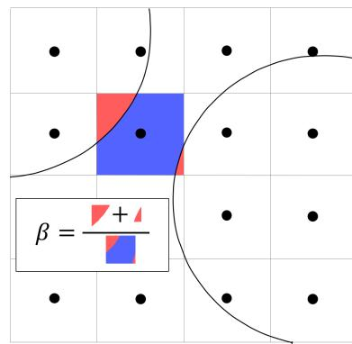
incorporates an additional solid collision operator,  $\Omega_i^S$ , and solid weighting function,  $\beta$ , into the discretised lattice Boltzmann equation The PSM fully recovers fluid-particle hydrodynamics, and as such efficiently captures the physics of individual particles at the spatial scale of a coal cleat.
