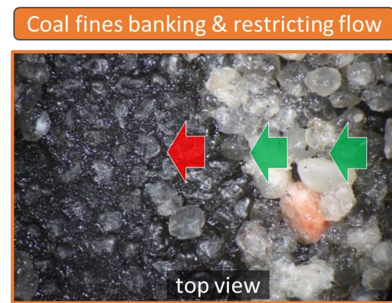
Microscopic images of sand embedment and fines generation in a HV Bituminous coal
