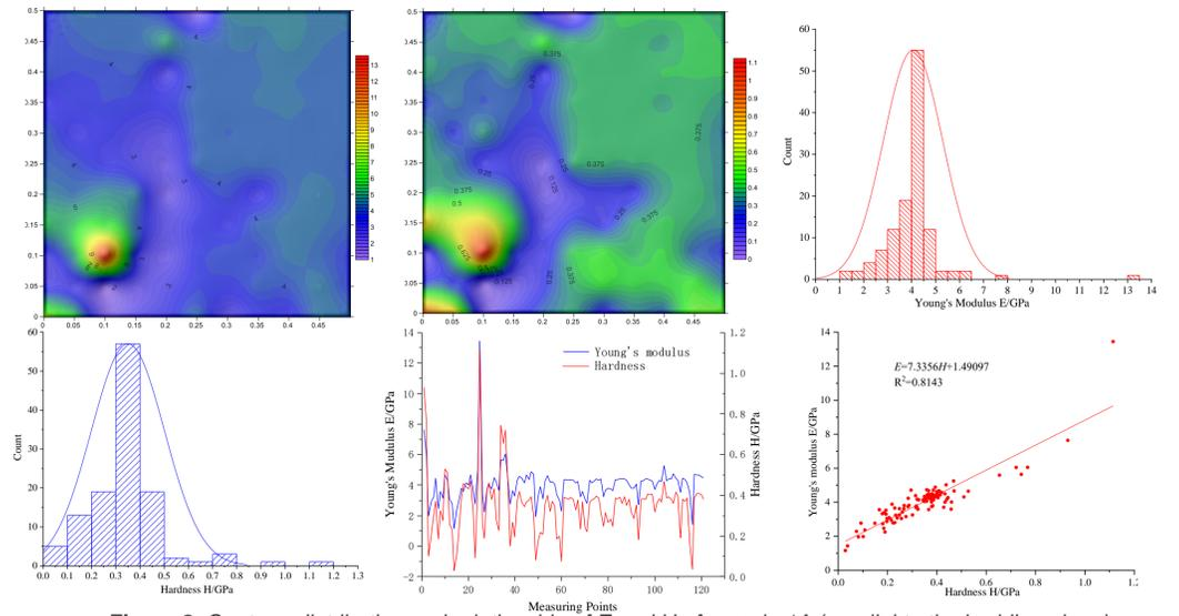
Figure 2: Contour, distribution and relationship of  $E$  and  $H$  of sample 1A (parallel to the bedding plane)
