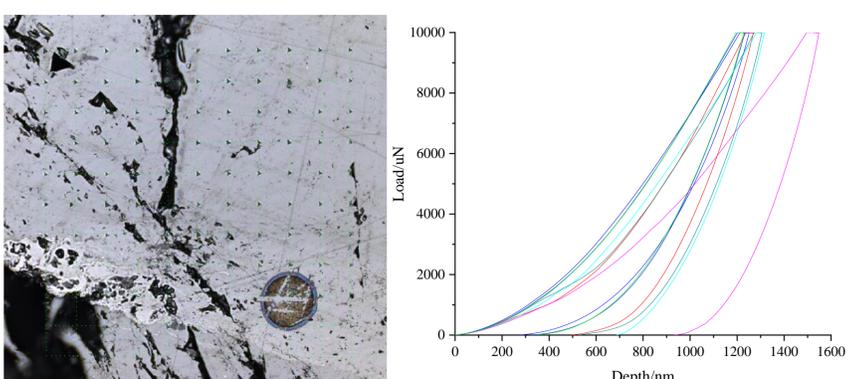
Figure 1: An indentation image (left) and load-depth curve
