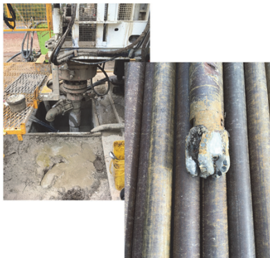
Fig 1: A 4 3/4" BHA was made up and the used to ream down the hole to 113.7m GL.
