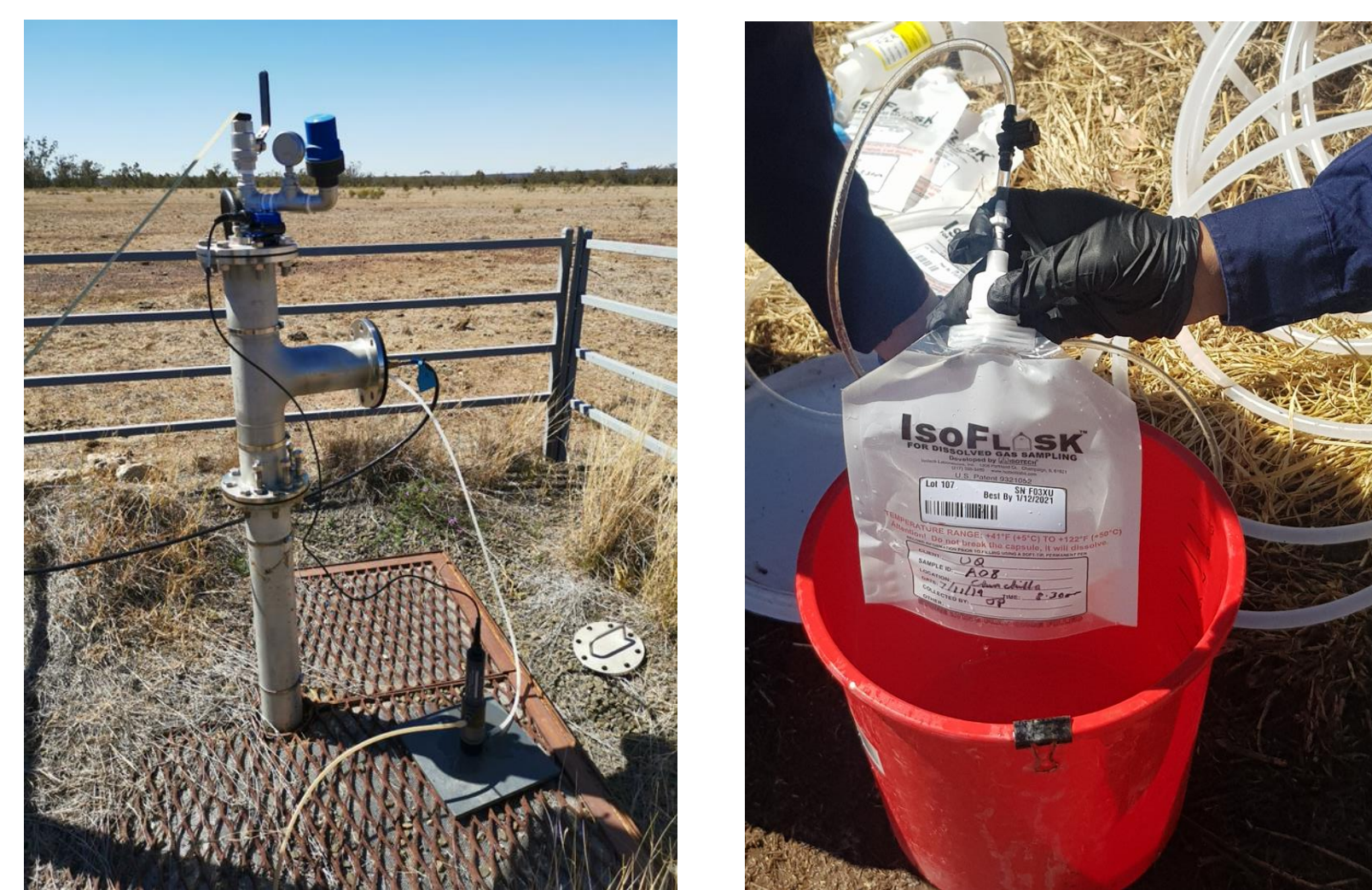
Figure 7: A monitoring bore being pumped, and sampling dissolved gas with a closed sampling method.
