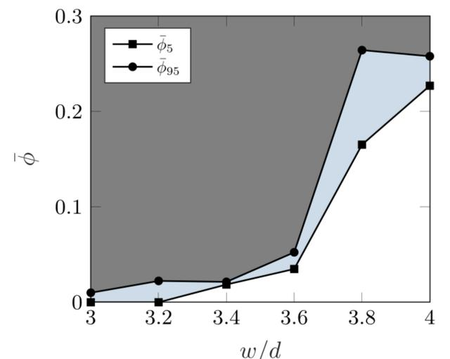
**Figure 5:** The influence of electrostatics on clogging. For  $w/d > 4$  no clogging occurs, while all values  $w/d \leq 3$  are equal.
