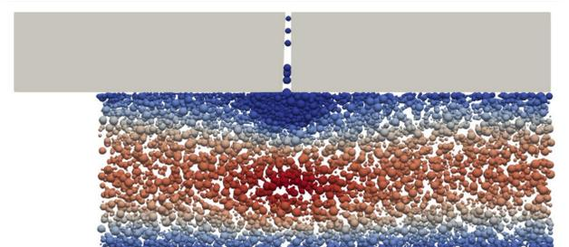
**Figure 5:** The formation of a proppant mound at the entrance to a 160 $\mu$ m cleat when a combination of 100 and 625 mesh is carried by a Newtonian fluid. The use of a shear-thinning fluid results in a smaller mound due to greater flow resistance (and therefore pressure drop) through the mound.
