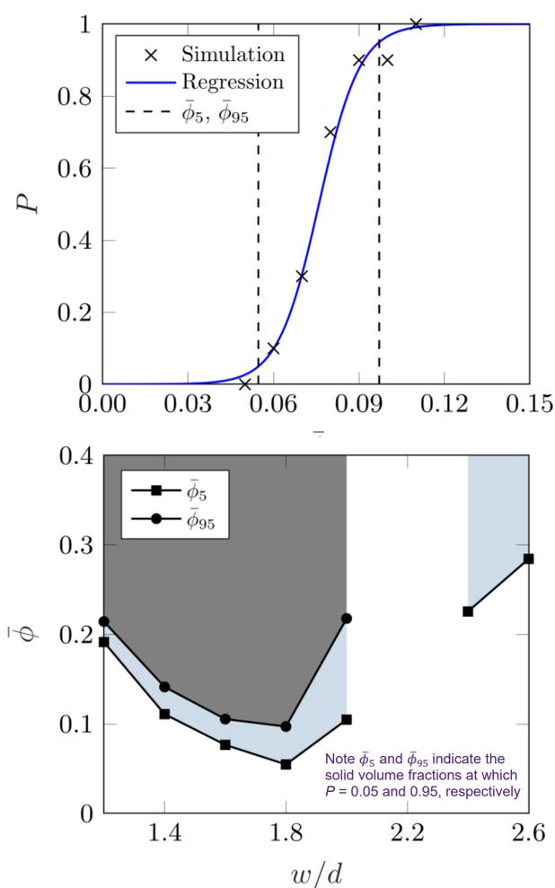
**Figure 4:** Results of proppant clogging analysis showing (above) a discrete set of clogging probabilities obtained via simulations and fitted with a predictive regression model ( $w/d = 1.8$ ,  $St = 0.1$ ), and (below) the dependence of clogging on the non-dimensional channel width,  $w/d$ .
