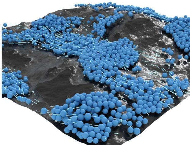
**Figure 1:** Rendered image of proppant transport in a synthetic coal cleat, as modelled using the lattice Boltzmann method (LBM) and discrete element method (DEM). The simulation framework includes non-Newtonian rheology and DLVO forces.
