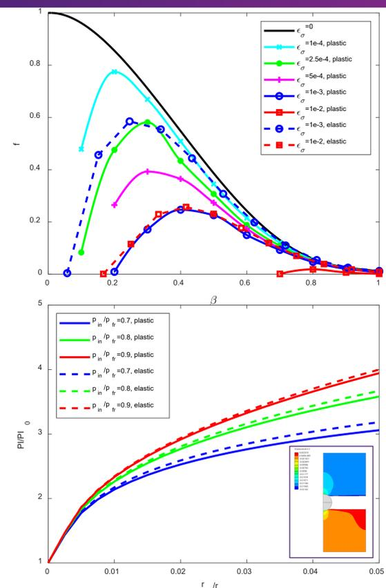
**Figure 2:** Results of proppant embedment analysis showing (above) retained fracture permeability factor,  $f$ , as a function of monolayer pack spacing,  $\beta$ , with and without (inset) elastoplastic coal deformation, and (below) the resultant productivity index,  $PI$ .
