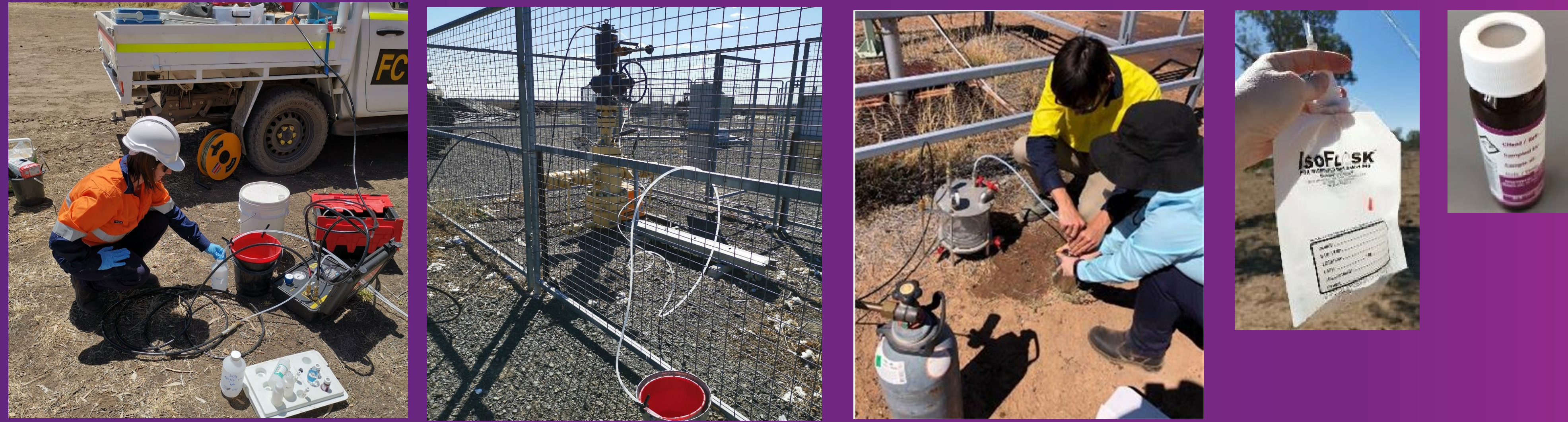
Figure 1: Sampling water bores in the Surat Basin. Showing the Terra Sana gas-water separator, Isoflask, and vial containers used for sampling methane.
