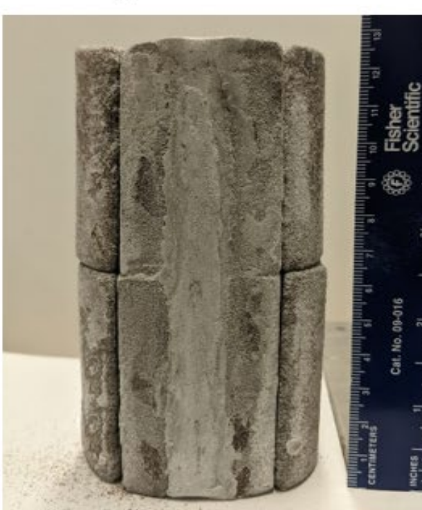
Figure 3: Photographs of synthetic rocks and histogram of permeability before and after treatment with sodium silicate and carbon dioxide.
