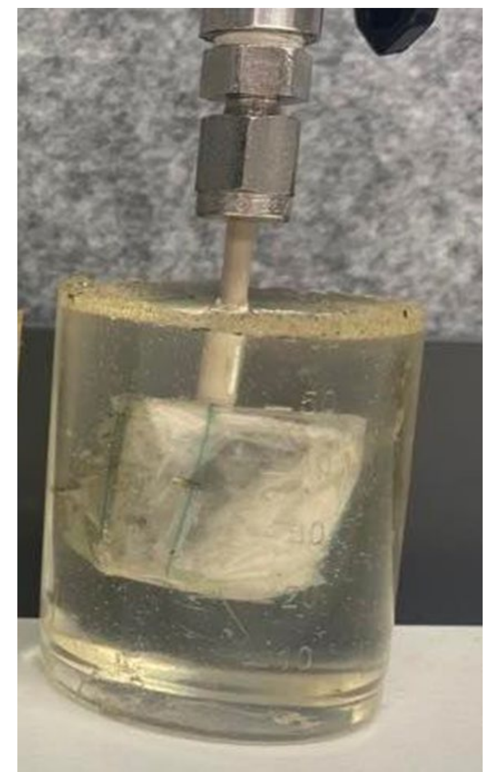
Fig 1: X-ray transparent device, showing coal and PEEK tubing set in resin. Tested to 700 psi
