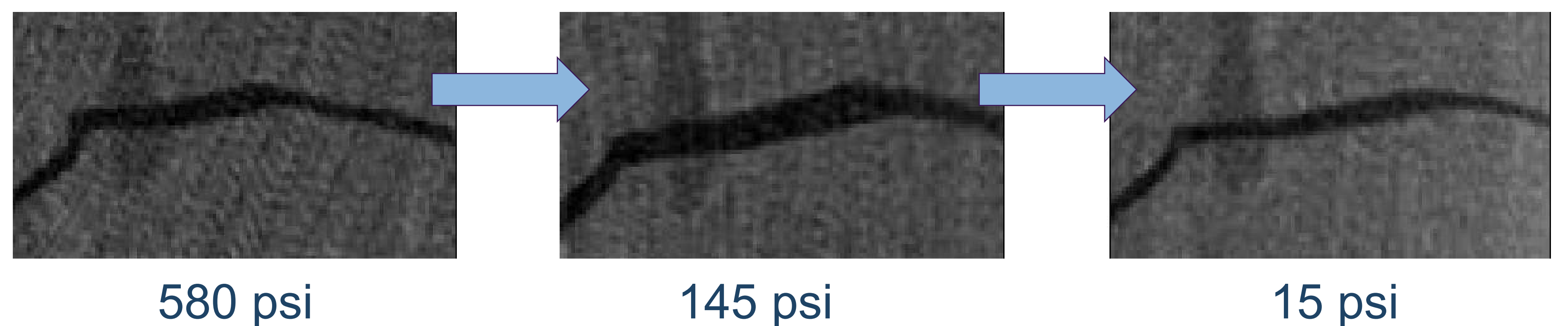
Fig 2: X-ray micro-CT scans (Surat coal, perpendicular cleat) showing increase in cleat porosity (by 32%) from 580 psi to 145 psi and decrease (by 11%) to 15 psi.
