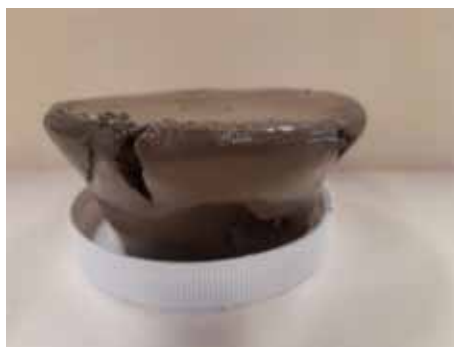
Figure 46. Formulation of “guar-gel+proppant” at 8 ppg 30 min after its preparation
