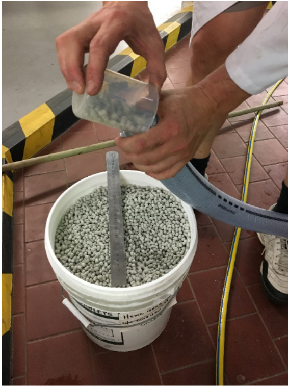
Figure 46: Loading compressed bentonite tablets into a 10m long 2" hose.
