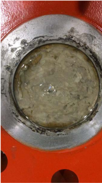
Figure 30: 5A-raw in a 4" pipe / fourth hydraulic test. Air bubbles occur at the center of the plug and at the interface plug/steel pipe at failure pressure.
