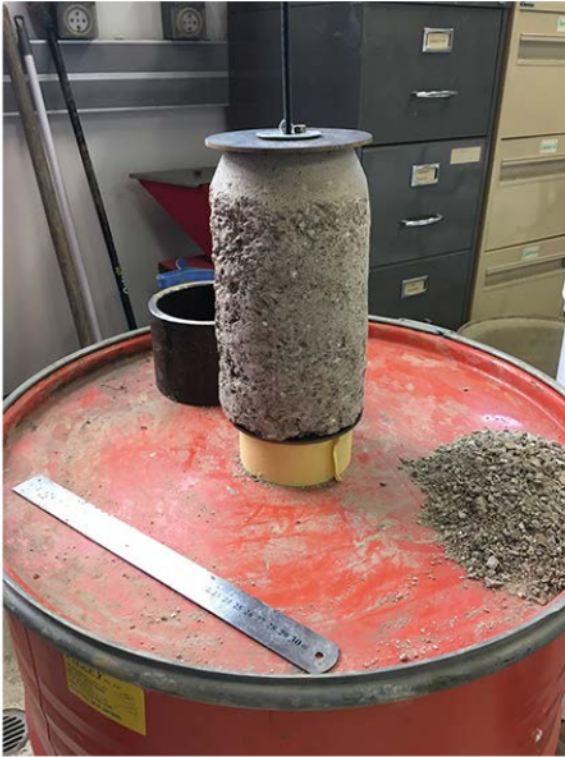
Figure 33: Originally, 5.5" diameter plug, stripped to 5" for the long term 6" pipe section testing.
