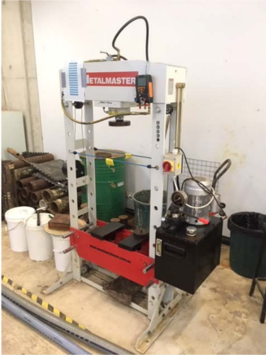
Figure 18: Industrial hydraulic Press used for primary mechanical dislodgment tests.
