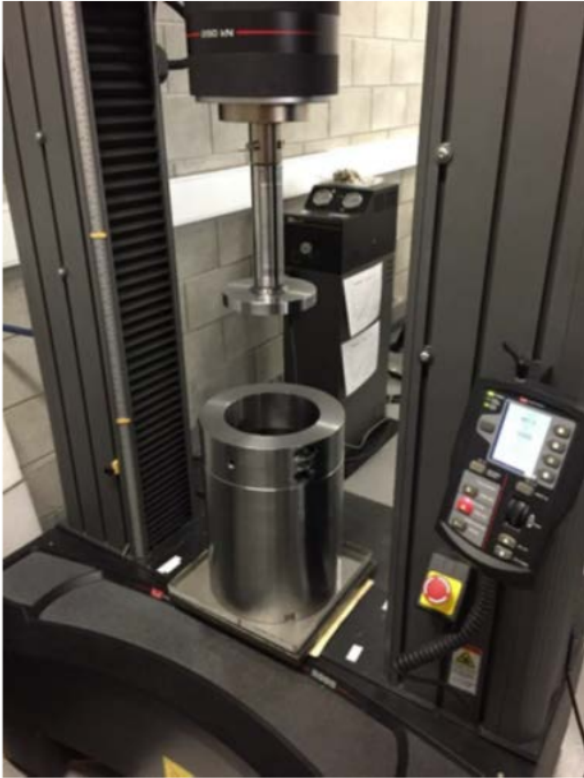
Figure 20: Instron 250 kN loading frame with steel clamp for central installation of the 80cm high 7" steel pipes.
