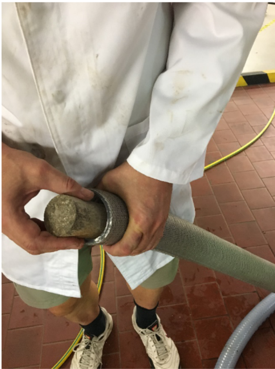
Figure 45: Placing of ten plugs into a 10m long 2.5" hose.
