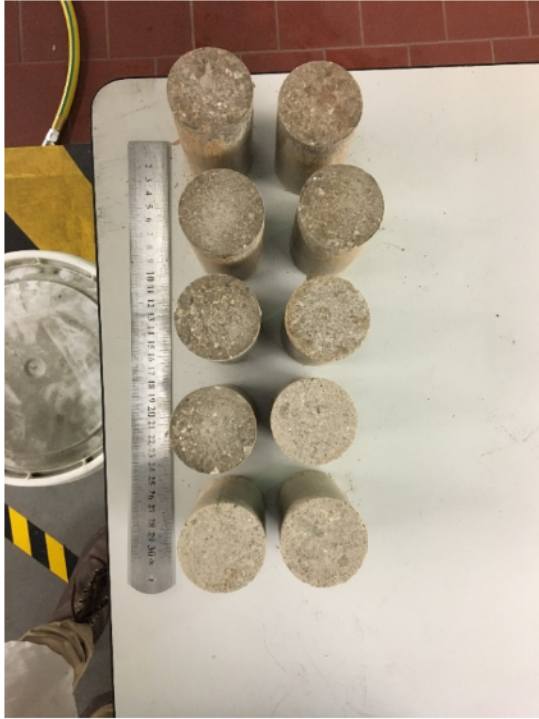
Figure 44: 2" diameter cylindrical plugs with a height of 10cm, compressed with 15t.
