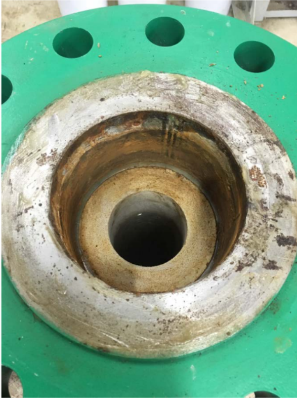
Figure 39: Helidon Sandstone Cylinder after hydraulic testing. The sandstone is installed in an 8" steel casing, using a high tensile and flexural strength, low viscosity epoxy resin.
