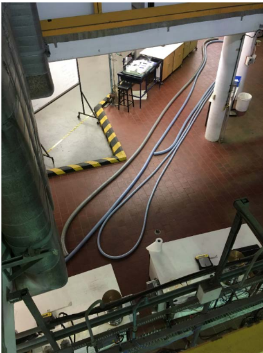
Figure 43: 20m sections of 2 and 2.5" ID translucent reinforced PVC hoses used for the pumping trials.
